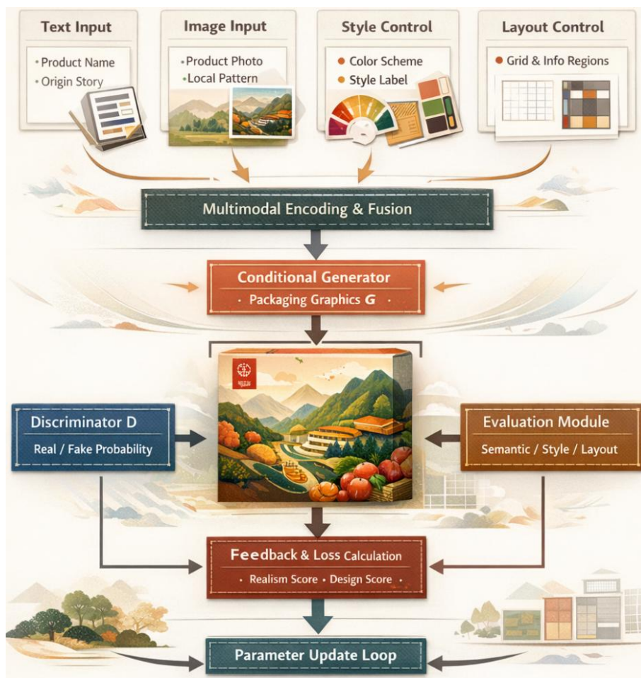
Figure 2: Process of packaging graphics generation and training based on multimodal AI generation technology
