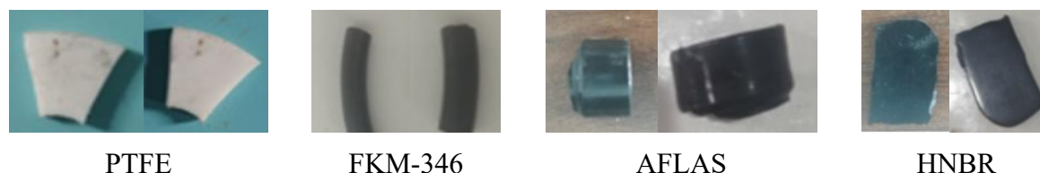
Figure 6: Comparison of materials appearances before and after corrosion
