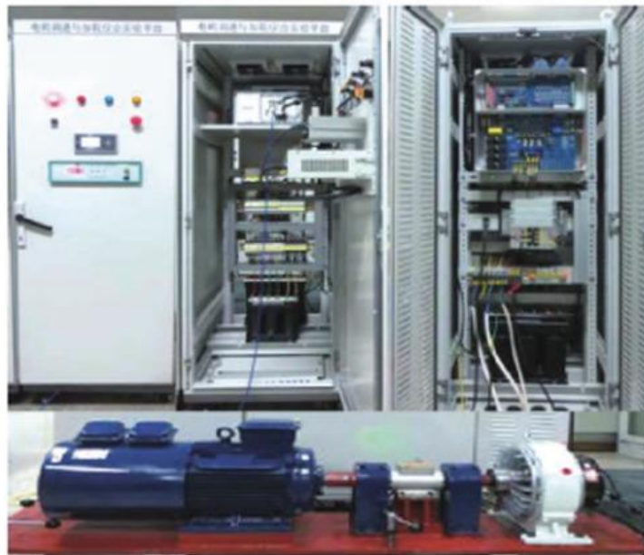
Figure 6: Photograph of the integrated motor drive and dynamometer loading testbed.
