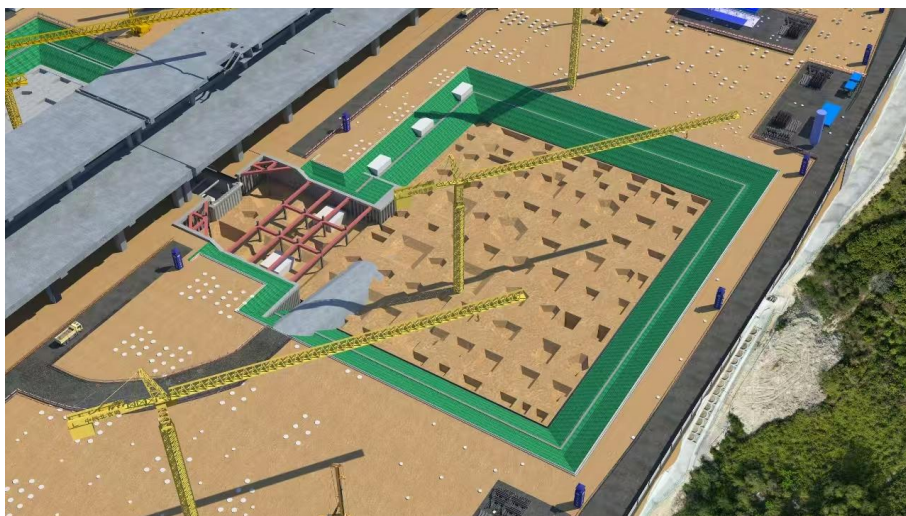
Figure 10: BIM Model for Construction Simulation
