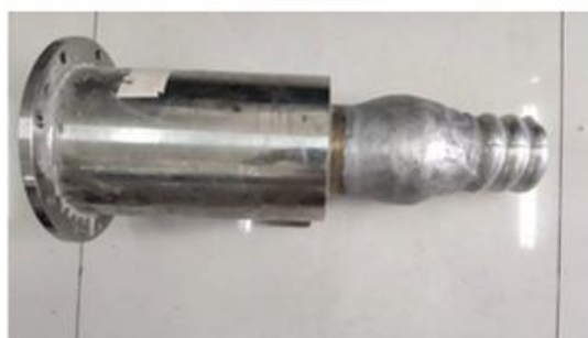
(b) Sample appearance of cable termination seal
