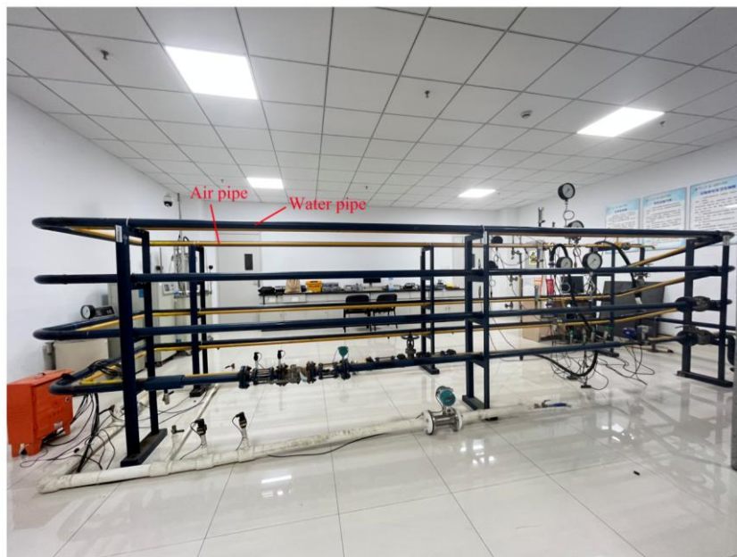
Figure 4: Pipeline Leakage Experimental Simulation Platform.
