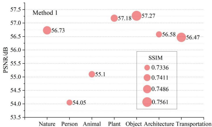
Figure 6: The PSNR and SSIM values of the AI images generated under Method 1
