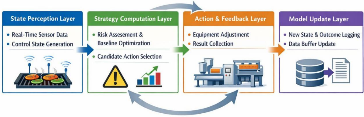
Figure 5: Closed-loop regulation strategy diagram of food processing process incorporating data-driven model
