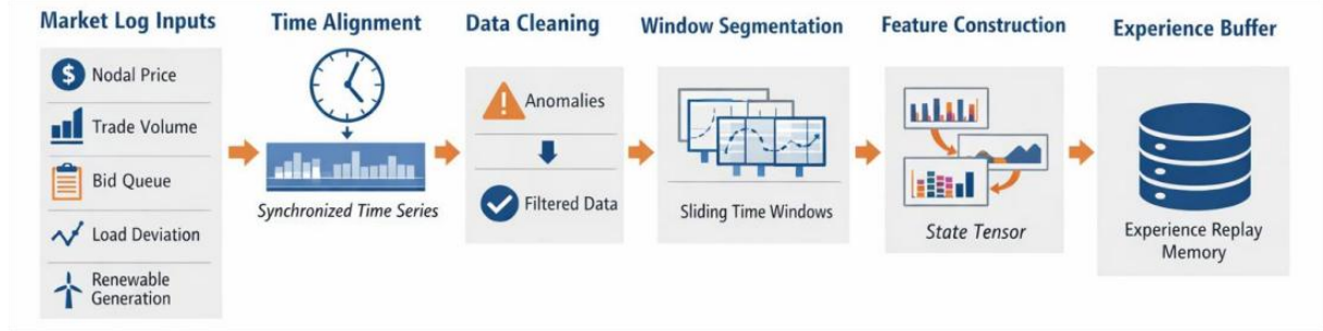
Figure 2: time series data organization and feature construction process of high-frequency trading in electricity market
