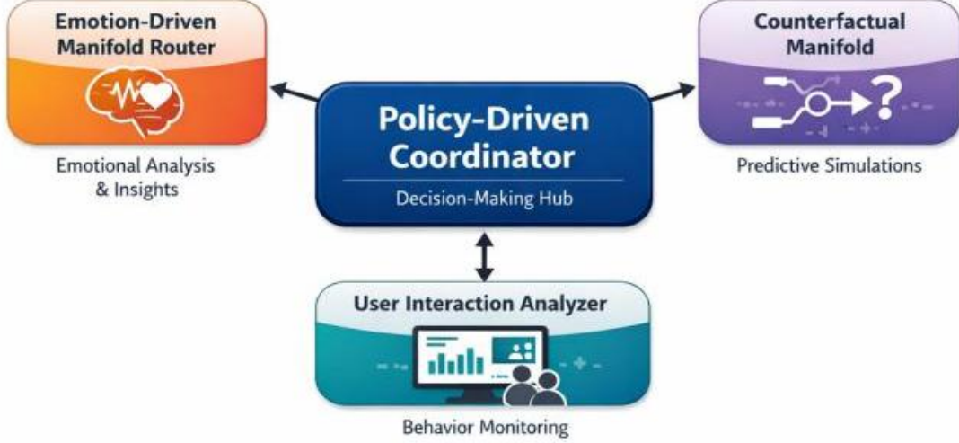
Figure 4: Schematic diagram of the Policy Driven Coordination strategy as a part of the Emotion Driven Manifold Router model. The Policy Driven Coordinator at the center combines the inputs given by the Emotion Driven Manifold Router, Counterfactual Manifold, and User Interaction Analyzer in order to maximize the recommendations of content. Such dynamic interaction makes it possible to predictively simulate, analyze emotions, and monitor behaviors in order to match the recommendation policies with the emotional state of the user and their behavioral patterns.
