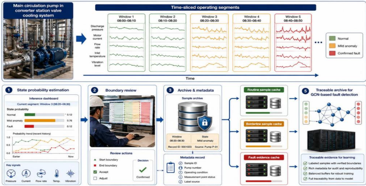
Figure 2: Anomaly state calibration and sample archive structure
