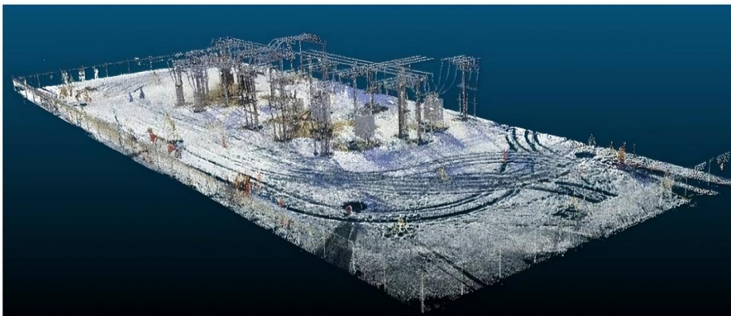
Figure 4: Typical example of point cloud data for substation components
