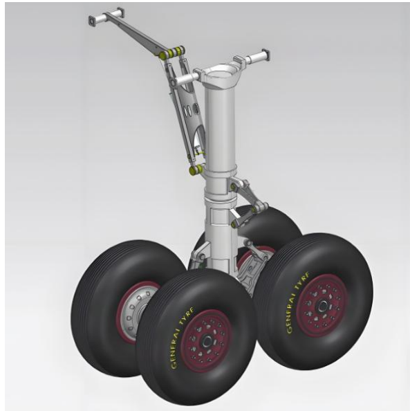
Figure 1: Single leg model of aircraft landing gear
