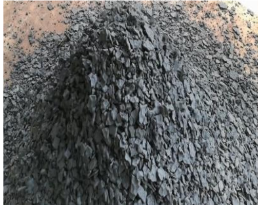
Figure 21: Diagram of sludge with a moisture content of 50% after drying
