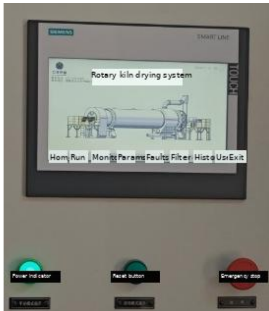
Figure 20: Touch screen control interface diagram of electric control cabinet
