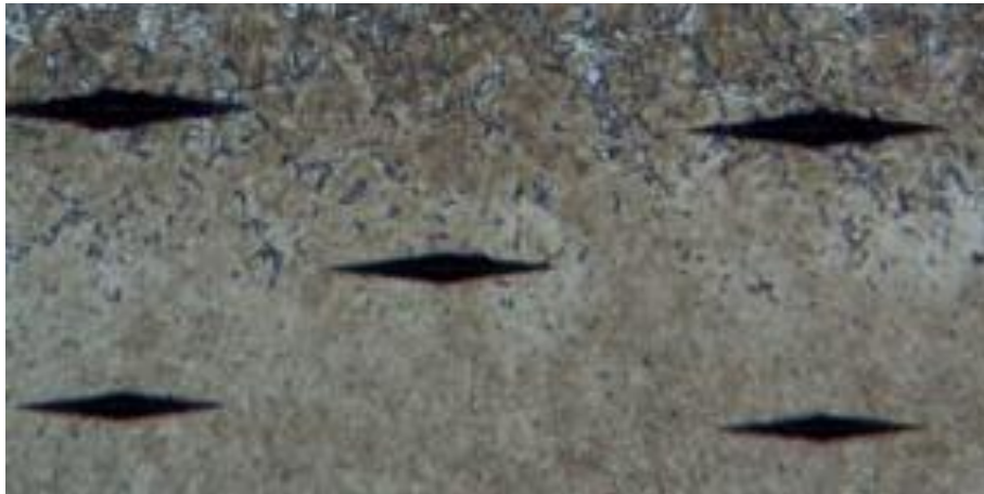
Figure 1: The micrograph of carburized 1215 steel containing “lip-shaped-crack-like” defects (Courtesy of Metal test Inc. and CES Engineering Guide.)
