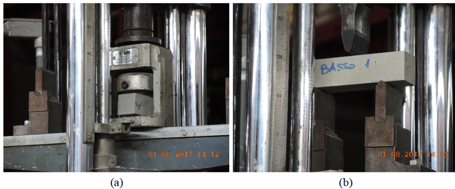
Figure 4: Photographs of the setup for (a) compression and (b) three-point flexural testing of mortar samples
