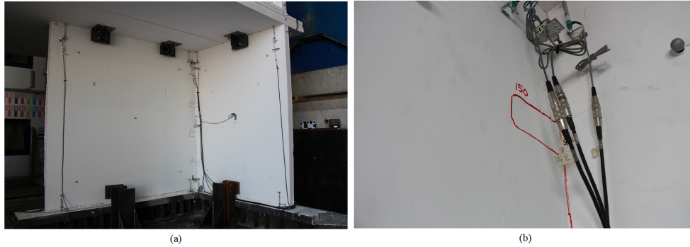
Figure 15: Damage mechanisms/patterns at the end of test run 150% (Brunesi et al. [8]): (a) full-depth cracks in the base wall joint and (b) example of cracks along the boundaries of the connectors' sockets
