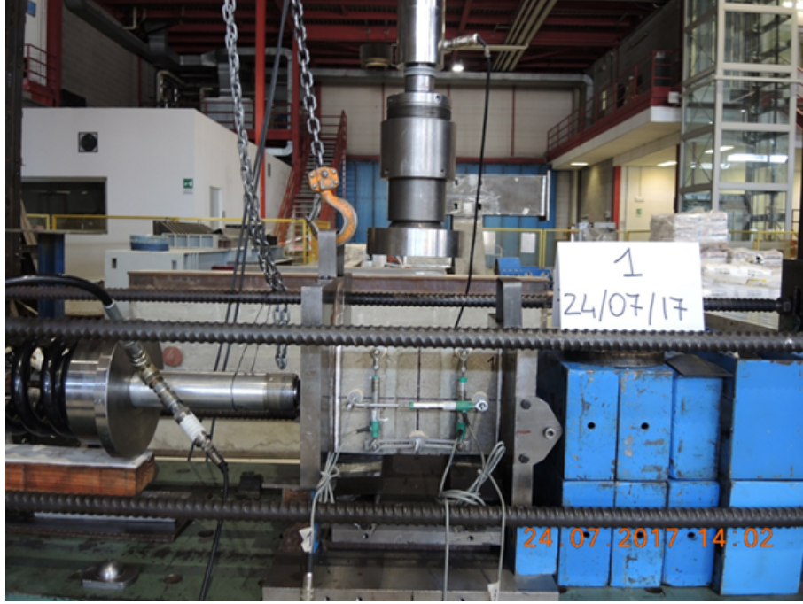
Figure 9: Example of concrete-mortar triplet specimen installed in the testing apparatus
