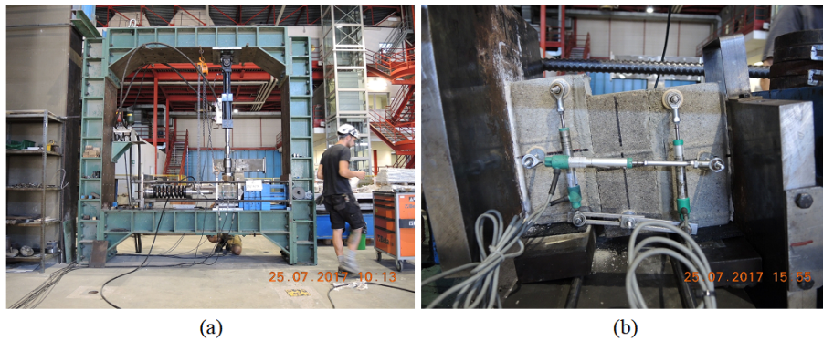
Figure 10: Friction testing of triplets: (a) test setup for application of vertical and horizontal forces and (b) triplet specimen at the end of the test
