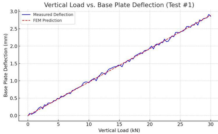
Figure 8: Vertical load vs. base plate deflection under static loading (Test #1)
