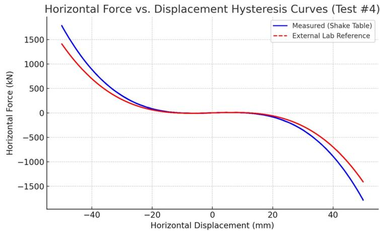
*Figure 11: Horizontal force vs. displacement hysteresis curves for the SSI prototype (Test #4)*
