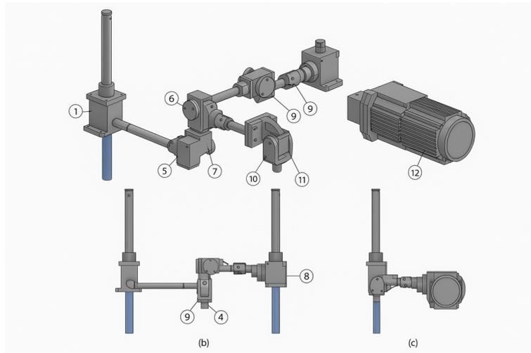
Figure 2: Mechanical diagram of the vertical load transmission system, showing screw jacks, shaft couplings, angular transmissions, and brushless motor assembly
