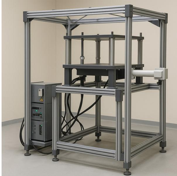
Figure 3: Photograph of the assembled shake table system, highlighting the actuator, guide-ways, structural frame, and control units
