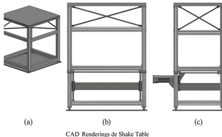
*Figure 1: CAD renderings of the shake table structure: (a) Isometric view, (b) Front view, (c) Side view*
