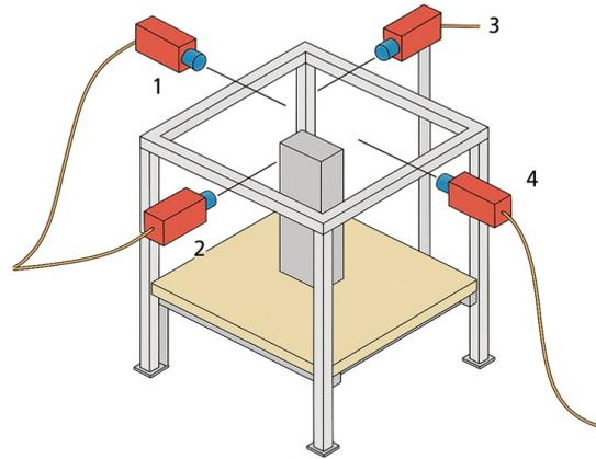
Placement of laser displacement sensors on the shake table and test specimen.
