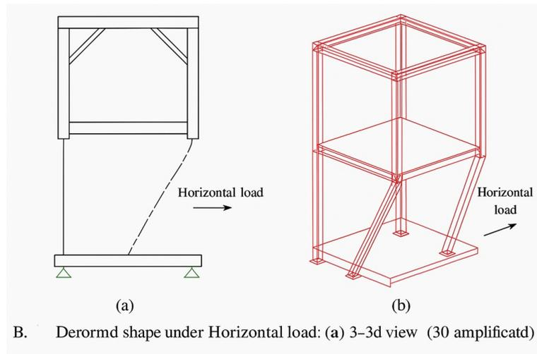
Figure 6: Deformed shape under horizontal load: (a) 2D elevation view, (b) 3D view (30% amplified)
