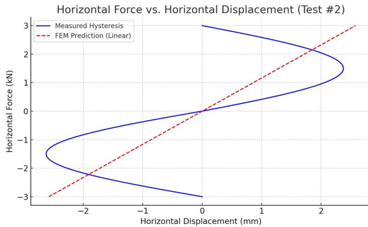
Figure 9: Horizontal force vs. horizontal displacement curves under lateral loading (Test #2)
