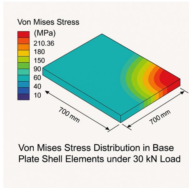
Figure 5: Von Mises stress distribution in base plate shell elements under 30 kN load
