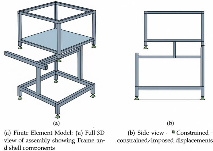
Figure 4: Finite element model overview: (a) Full 3D view of the assembly showing frame and shell components, (b) Side view with boundary condition annotations
