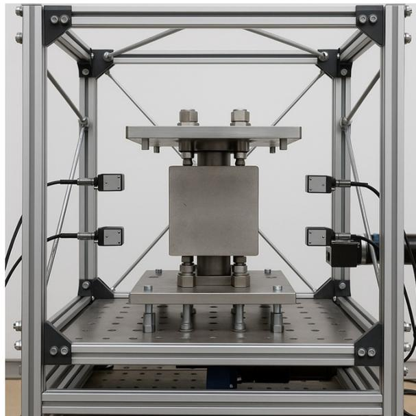
*Figure 12: Views of the SSI prototype installed on the shake table for dynamic testing*
