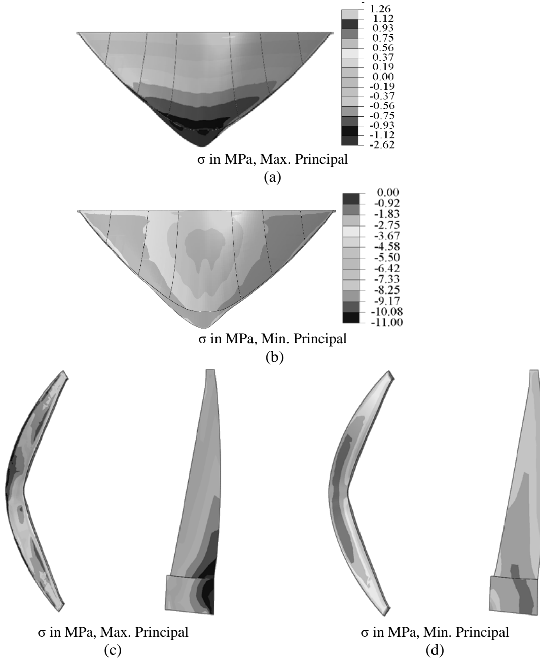
Figure 9. Principal maximum and minimum stresses for DM1982 case 04. (a-b) upstream face, (c) pulvino and (d) crown cross-section
