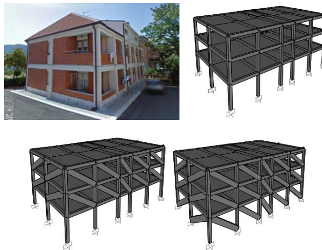
Figure 8 – Example of the structure modelling for the 3 considered infills configurations. Clock-wise starting from higher left: image of the building typology, bare frame, completely infilled and pilotis configuration models.
