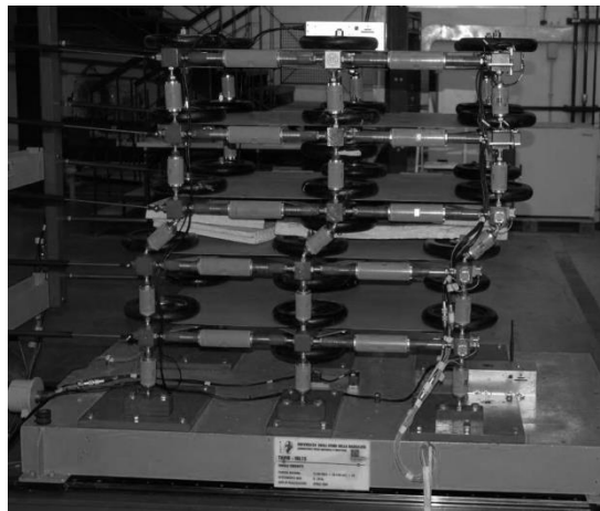
Figure 25. Mechanism pillars plasticized on the third floor of the model so as estimated by the method for damage localization (Ponzo et al., 2014)
