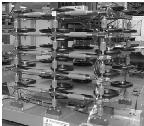
Figure 13. Frontal and lateral visualization of the shaking-table and the five floor 1:15 scaled structure (Ponzo et al., 2014)
