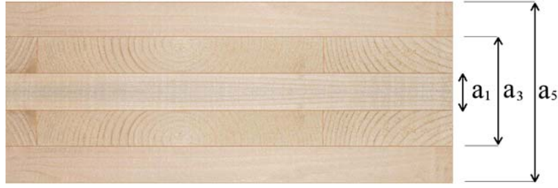
Figure 9. Definition of various thicknesses in a generic 5-layer CLT panel
