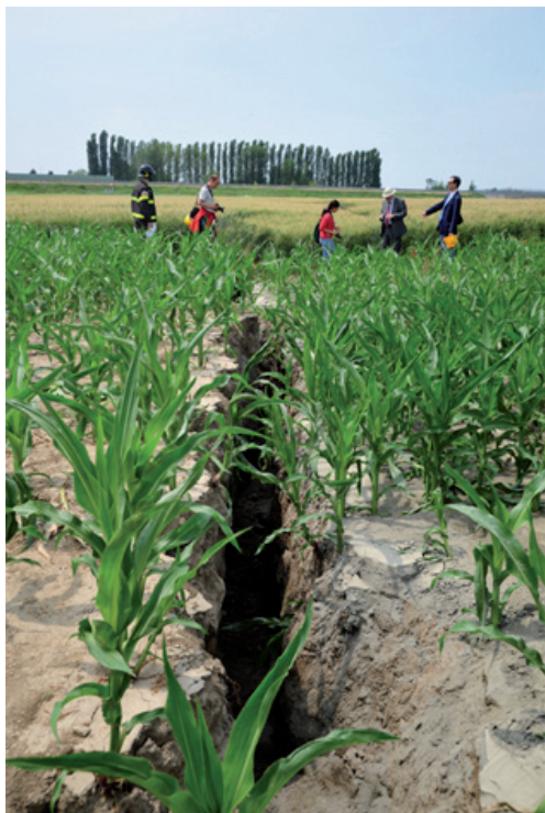
Fig. 11. ENE-WSW trending lateral spreading and liquefaction in San Carlo. Estimated ground crack length 300m. Maximum opening of 1m and vertical offset of 0.5m.
